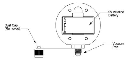
Rear View (Battery Cover Removed)
